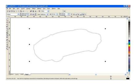
C1-5.2 Ensure that the paper size is set correctly by selecting the AAS paper size if the AAS hardware is installed on the machine. Note that by selecting the AAS paper size, the working area will be capped to the maximum working area of the laser engraver with the AAS system installed.
