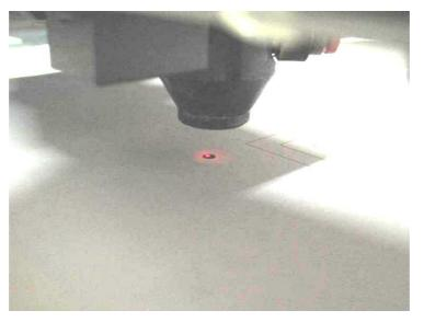
C.1-8 Press "Start" on the control panel of the LaserPro machine, and the AAS module will identify the position marks and contour cut the graphic with precision
